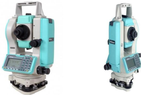
Figure 1. Total Station Nikon DTM – 322[10]
