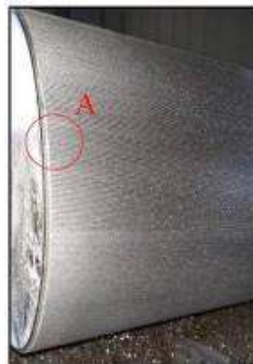
Figure 12. Fluted Roll Surface After Passing Scraping Process
