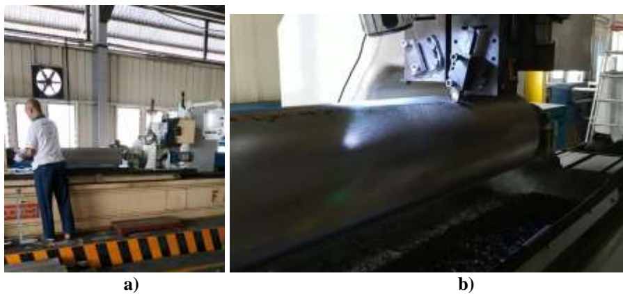
Figure 11. a)CNC Machine Used For Scrap Process, b)Roller Mill Scrap Process into Fluted Roll
