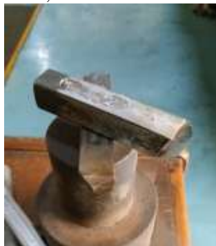
Figure 7. High-Speed Steel (HSS) Chisel Used in the Fluted Roll Scrap Process
