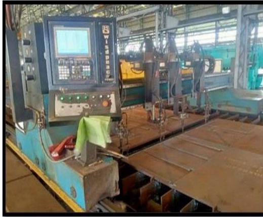
Figure 1. Plasma Cutting Machining Process
