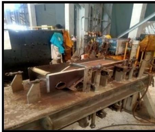
Figure 12. Tack Welding and Welding Process in Bolsters
