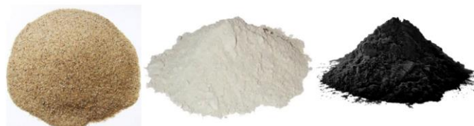
Figure 2. Material of Molding (Silica Sand, Bentonite, Sea Coal)
