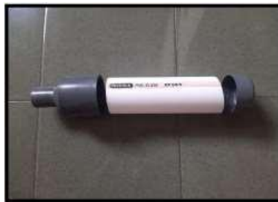
Figure 2 PVC pipe Battery storage
