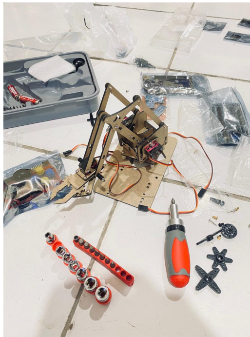
Figure 2. Assembled 3-DOF robotic arm system showing mechanical structure and servo motor placement
