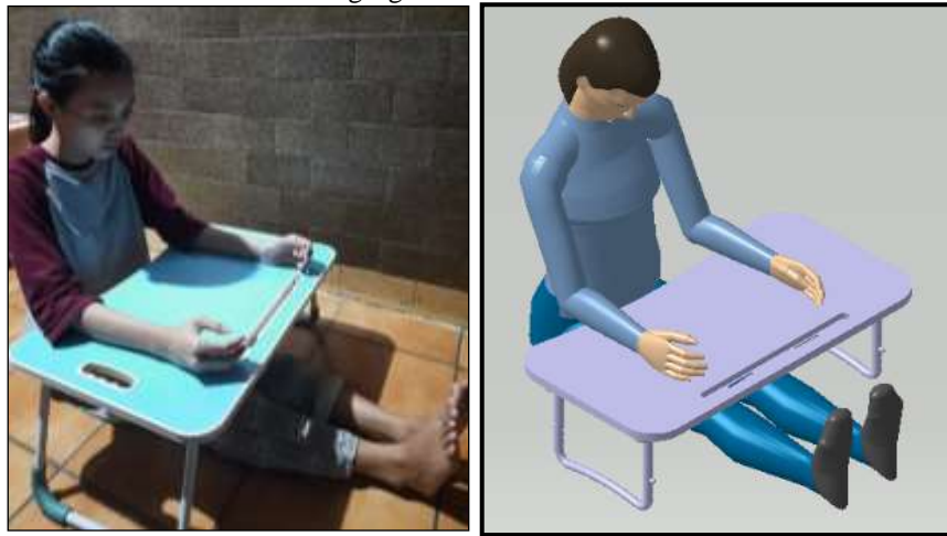
Figure 3. Mannequin Position For Simulation Risk Posture User of a Fortable Study Desk
