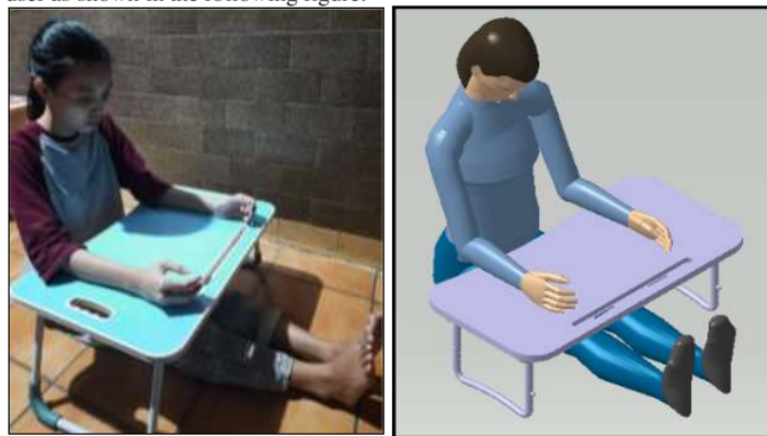
Figure 3. Mannequin Position For Simulation Risk Posture User of a Portable Study Desk
