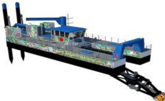
**Gambar 1.2. Cutter – Suction Dredger**
