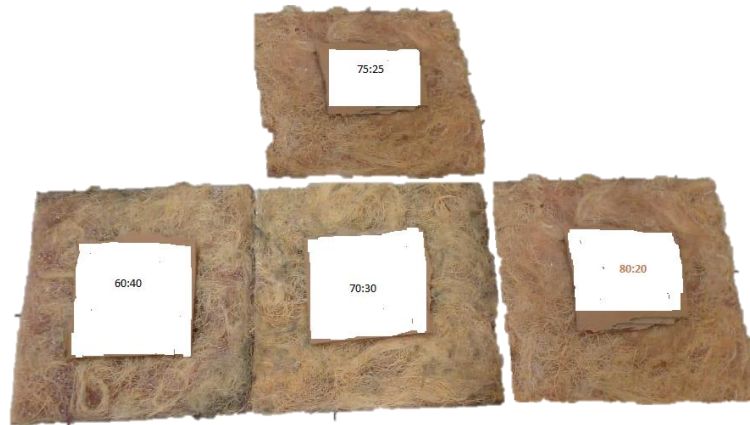
Figure 2. Composite board made from sugarcane bagasse mixed with resin
