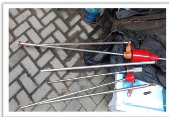
Gambar 2. Alat Dynamic Cone Penetrometer (DCP)
