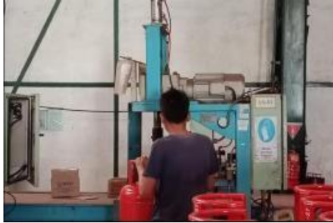
Gambar 6. Pemasangan Valve Screw
