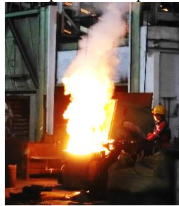
Gambar 8. Proses Mg treatment
