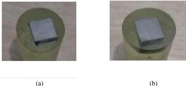
Gambar 2. Foto specimen tanpa perlakuan (a) specimen menerima perlakuan pack carburizing (b)
