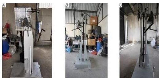
Gambar 3.3 Alat Uji Impact Charpy
