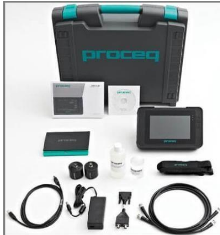
Gambar 6. Alat UPV Pundit Versi Digital Sumber: Testindo, 2022
