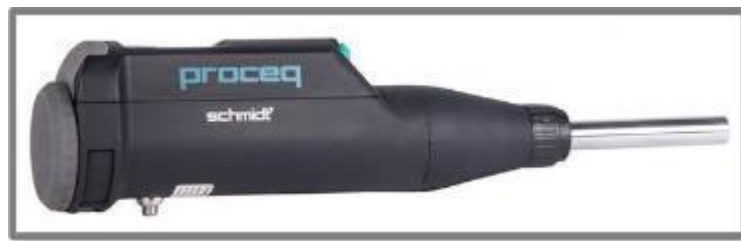
Gambar 8. Schmidt Rebound Hammer Live Digital
