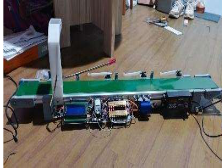
Figure 3. Physical prototype of the conveyor-based sorting system and sensor/actuator placement.
