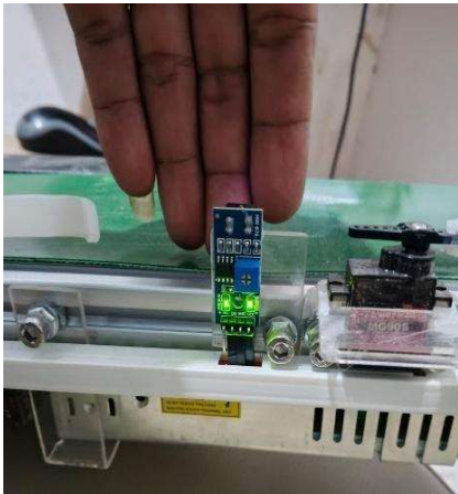
Figure 5. Infrared Sensor is used to illustrate the IR sensor implementation on the conveyor prototype.
