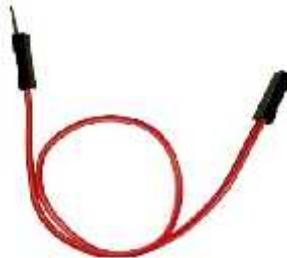
Gambar 2.8 Kabel Jumper Male to Female
