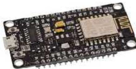
Gambar 2.2 NodeMCU ESP8266
