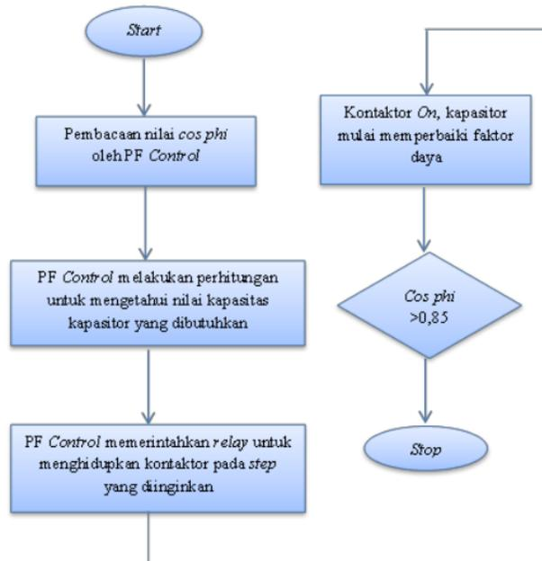
Gambar 7. Bagan Sistem Panel Kapasitor Bank 1200KVAR
