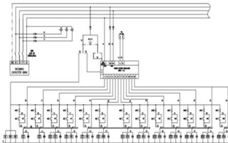
Gambar 6. *Wiring Diagram* Panel Kapasitor Bank 1200 KVAR
