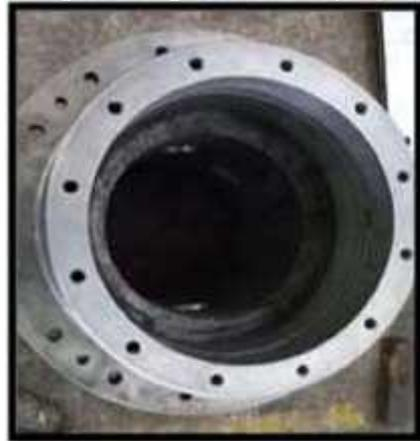
Gambar 10. Hasil Proses Grinding
