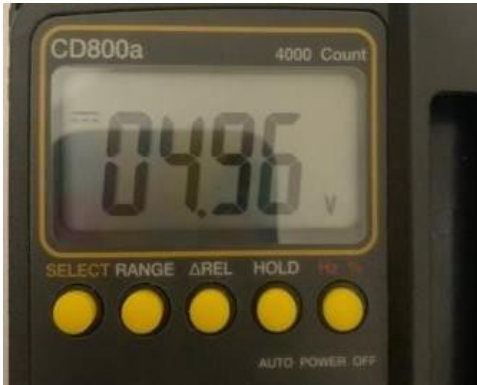
Figure 6. TP3 Voltage Measurement Procedure
