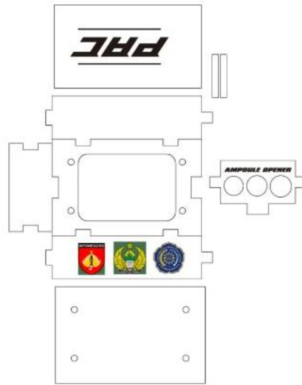
Figure 1. 2D Prototype Design of PAC (Pocket Ampoule Cutter)
